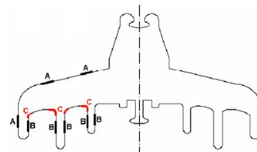
Fig. 1. Sampling points along the insulator coated surface for the coating thickness measurement.
