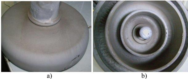
Fig. 2. Visual inspection: a) insulator #12 top surface with a lateral scrape; b) insulator #1 bottom surface with dirt under ribs and without interesting signs of degradation.
