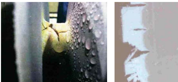
Figure 6 : silicone rubber degradation related to acid and detailed cross section.
