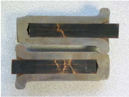
Figure 4 : crack in the rod after excessive or uneven crimping operation. The crack is far enough inside the end fitting to go through the mechanical routine test without being detected.
